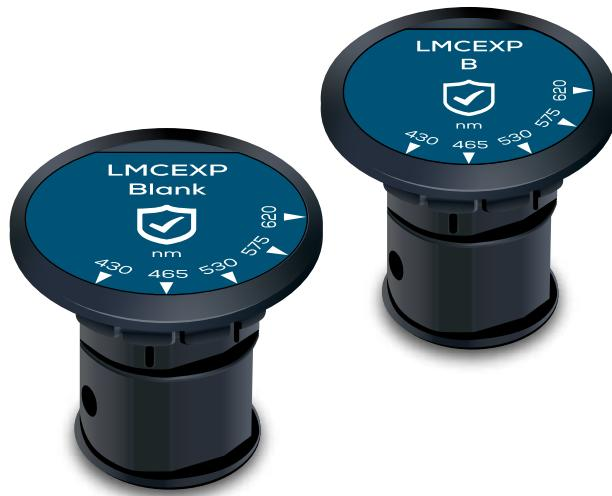
Using check standards is a simple way to verify the performance of the instrument and check that it is within calibration.
